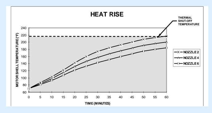
The motor driving this pump has a built in thermal protector that will open, shutting off the pump, when the surface temperature of the motor heats to approximately 215°F. Motors of this size and construction require 15 to 30 minutes of cooling time before the thermal protector closes and re-energizes the pump. Lower current levels heat more slowly, allowing longer run times, but the cool down time still averages about 30 minutes, at 70°F ambient temperature.
