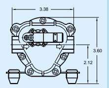
Series 5800 Pump Floor Care Applications 115 VAC Operation 3/8" NPT Female Ports Pressure Switch Set to 220 PSI Internal Pressure Bypass Sealed Motor to Prevent Moisture Intrusion Steel Mounting Plate (Other Types Available)
